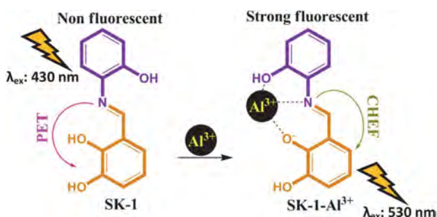
Fig. 8. Proposed binding mechanism between the compound SK-1 and \text{Al}^{3+} .
