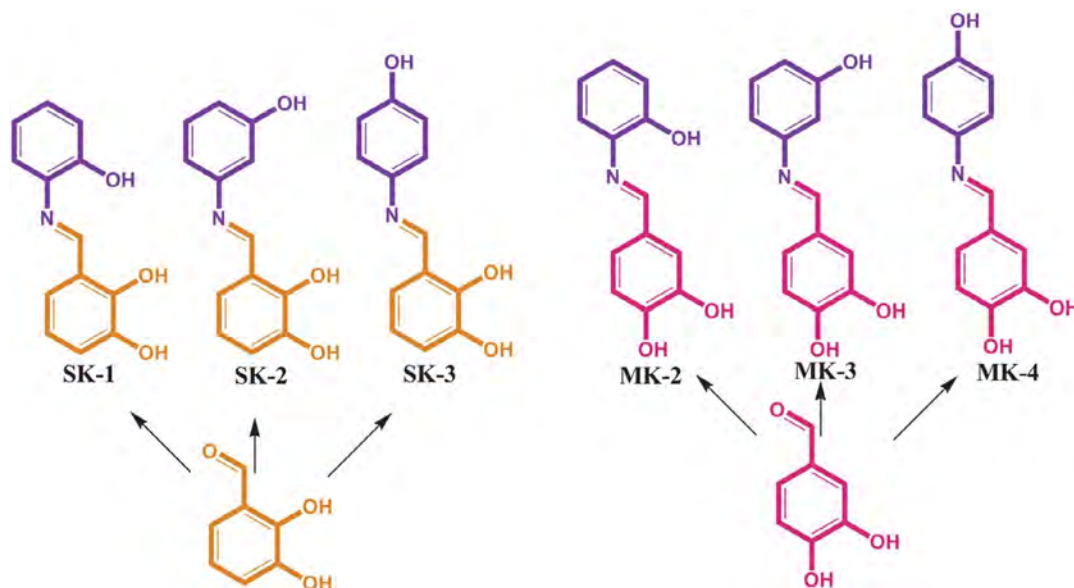
Scheme 1. The synthetic route of Schiff base compounds ( SK-1 , SK-2 , SK-3 , MK-2 , MK-3 , and MK-4 )
