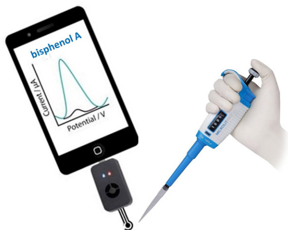
Figure 2. Portable sensing platform using all-in-one screen-printed electrode, hand-held commercial potentiostat, and smartphone.
