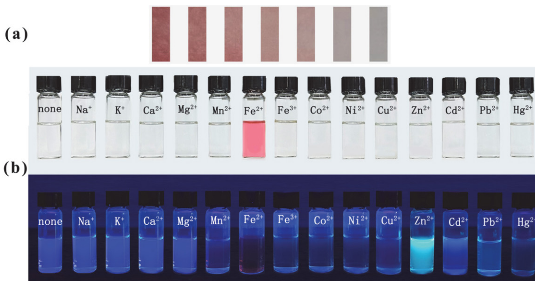
Figure 2. (a) Photograph of 1 test strips wetted by solutions containing 1.0 \times 10^{-2} , 5.0 \times 10^{-3} , 1.0 \times 10^{-3} , 5.0 \times 10^{-4} , 1.0 \times 10^{-4} , 1.0 \times 10^{-5} , 0 M of FeCl 2 (from left to right). (b) Photograph of 1 (50 \mu M) in EtOH-HEPES buffer (1:1, v:v, pH 7.2) solutions containing different metal cations (1 equiv) under visible light (upper row) and UV lamp (lower row).
