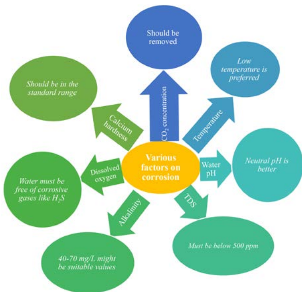
Figure 1. Effective factors and their conditions for preventing water corrosion and fouling
