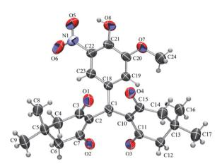
**Figure 6.** ORTEP-3 drawing of a molecule of **2** with the atom numbering scheme. Displacement ellipsoids are drawn for the probability of 50% and hydrogen atoms are shown as spheres of arbitrary radii.
